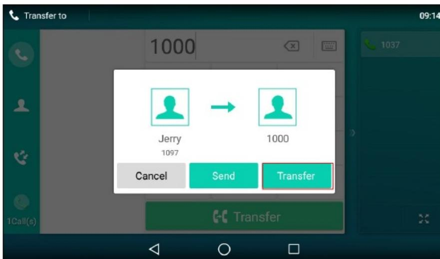
Select **Transfer** to complete the transfer (The call will automatically dial out in about 5 seconds if you do not select **Transfer**).
